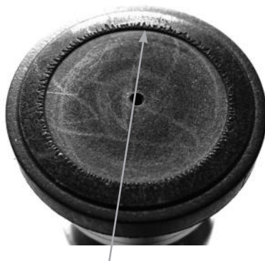
Cavitation of the piston shoes. New inspection is required in 3,000-4,000 hours.
